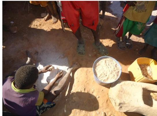
Fig 9- Crushing the quartz into powder
