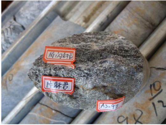
Fig 15- Amphibolite and gneiss rock in the boring core
