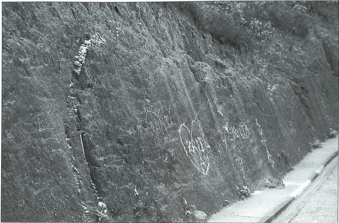
Photo 1 - The Zone of Corestone-free Weathered Rock (Zone I) with an Upper Creep Layer Indicated by the Curved Quartz Vein. Tai Tam Reservoir Road, Hong Kong Island (83905 81340).
